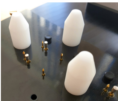
Figure 6: 1000A pulse with one needle per contact.
